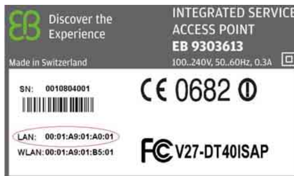
Fig. 73: Reading off the ISAP LAN MAC address
