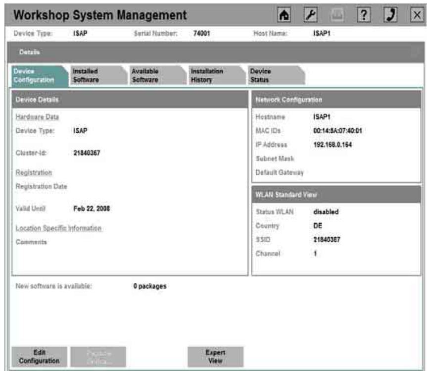
Fig. 138: Displaying the device configuration of the ISAP
