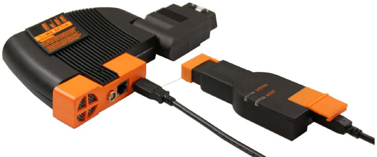
Fig. 10 Connection of ICOM A with B
