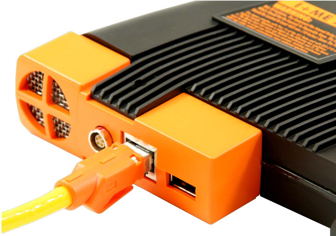
Fig. 5 Ethernet connection ICOM A
