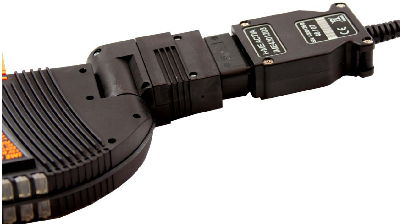
Fig. 14 Connection of ICOM A with C
