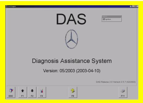
The DAS simulation mode allows you to access control unit-specific data without actually communicating with a vehicle or a control unit. When required by the test program, the ignition can be switched on and off in a separate window.
