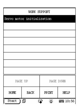
After clicking FUNCTION MENU, the screen will display the Process 1/3 Menu. It will prompt you that: If you want to change actuator, ECU and remove battery, please do this operation. Press 'YES' to do servo motor initialization. Press 'NO' to exit.
