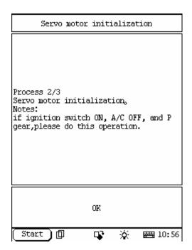
After confirming this operation, the screen will display Process 2/3 Menu: servo motor initialization. Note: please do this operation with ignition switch ON, A/C OFF and P gear. After satisfying these conditions, press OK to enter Process 3/3 Menu: [servo motor initialization] begin. After DEF blinking indicator turn OFF, press OK, then this operation is finished.
